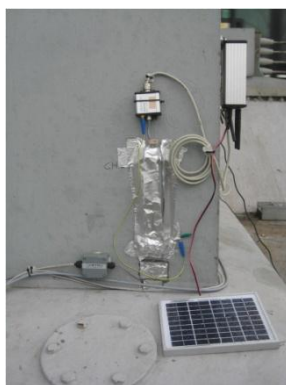
Figure 9 – «SENSKIN» sensor, solar cell, data modules are placed on the surface of the bridge pylon
